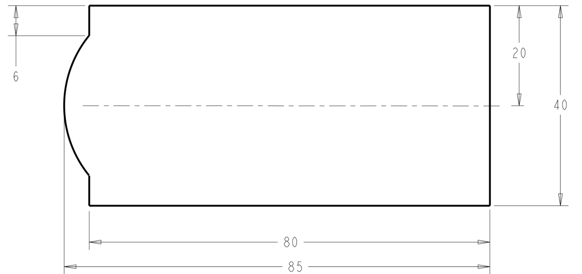
ITEM 3 - BASE PLATE MATERIAL - MILD STEEL NTS
